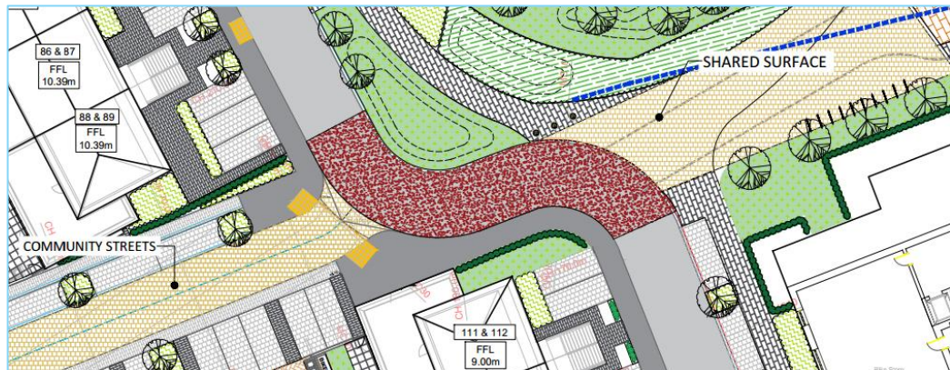
Figure 2-4 – Surfacing and Lack of Crossing Facilities at Junction 6
